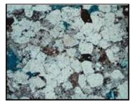
Conventional sandstone (left) has well- connected pores (dark blue). The pores of tight gas sandstone (right) are irregularly distributed and poorly connected by very narrow capillaries (NETL, 2011b NPR).
