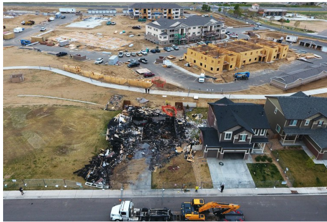
A gas well, seen in the upper left below the bike path, lies less than 200 feet from a Firestone, Colorado, home that exploded in late April, killing two. Investigators say the cause was a “fugitive gas leak” from an abandoned flow line that had been cut but not capped.
